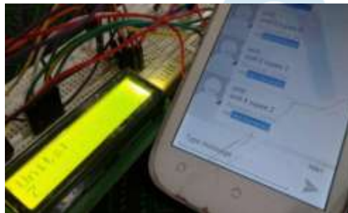
Fig 3: LCD displaying the total units consumed and the SMS of the bill
